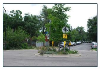
A traffic circle consists of a raised curb area installed in the middle of an intersection that requires drivers to travel around the obstruction as they enter the intersection. This is similar to the concept of a roundabout, but with a smaller footprint and slower speeds, as appropriate for neighborhood intersections.
