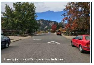
Speed bumps are additional asphalt with a substantial vertical deflection (i.e., a bump) installed across the width of the roadway that forces drivers to slow down to travel over. Speed bumps are generally installed in series along a roadway. Studies have shown that speed bumps installed at spacings of 260 to 600 feet provide optimal speed reduction along the length of a roadway.
