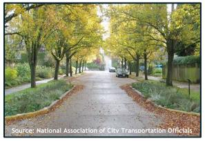
A pinch point is a series of two curbed areas on the edge of travel lanes that narrow the usable travel width to only allow for one-way traffic. This slows drivers to navigate the one-way section and also may convey the roadway is a local, slow-speed road.
