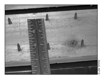
Use full or half sheets of the thickest plywood available. Nails should be long enough to stick out of the wood  $\frac{3}{4}$  - 1". Nails should be nailed into the board approximately 2" apart. Drawing a grid on the board makes it easier to stay on track.
